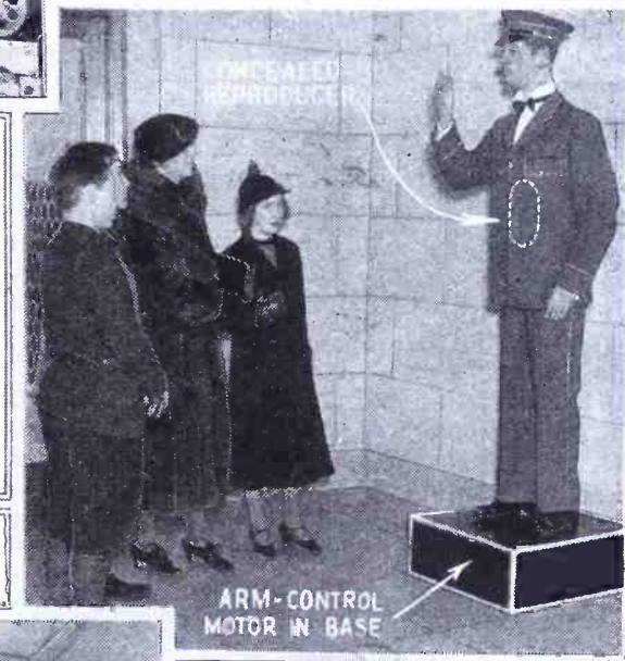
↑ This is Egbert, the electrical robot at the Benjamin Franklin Memorial, Phila., Pa. It is used to welcome visitors to the hall. A phonograph is the source of Egbert's voice and a relay under him operates a motor which raises and lowers his arm. A loud-speaker is located in his chest, and is the outlet for his voice. P.E. cells are connected to relays so that a person entering the building will set the mechanism in operation. Egbert tells you to have an enjoyable visit at the exhibition hall.
